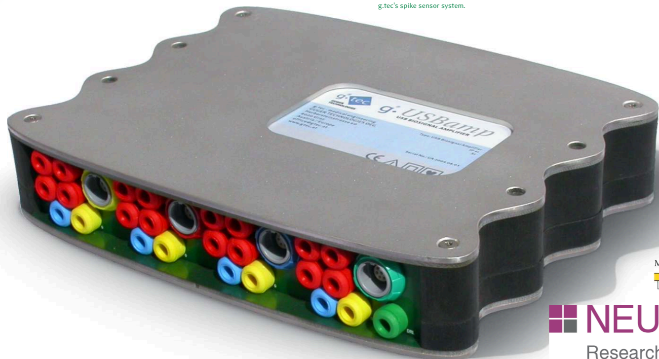
g.USBamp works with any type of passive electrodes and strip or grid ECoG electrodes. The g.GAMMASys active electrode system can be used as well. Single cell recordings can be performed in combination with g.tec 's spike sensor system.
