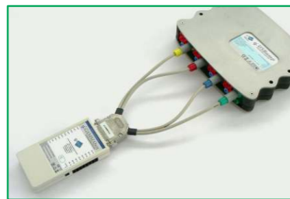
g.USBamp works with any type of passive electrodes and strip or grid ECOG electrodes. The g.GAMMASys active electrode system can be used as well. Single cell recordings can be performed in combination with g.tec 's spike sensor system.
